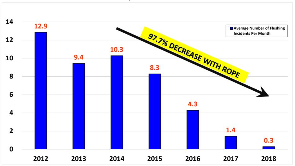
97% Reduction in Flushing Incidents when the Guideline Rope is Installed
